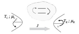
FIG. 1. A schematic representation of our model system. Electron transfer between the metals is blocked, but energy current is flowing through an excitation or deexcitation of the intermediate anharmonic (two-state) quantum system. The curved arrows represent energy transfer processes between the leads and the intermediating subsystem. In our work here we set  $\mu_L = \mu_R$  and take  $T_L > T_R$ .
