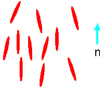
Figure 1.2: Most of the molecules are nearly in the same direction in the nematic phase [5].
