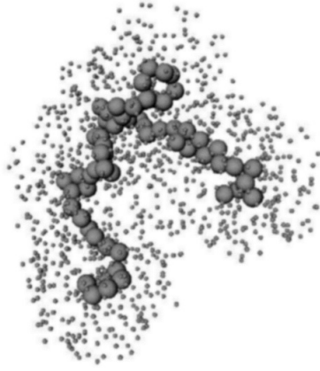
Fig. 15. Snapshot of a chain configuration showing a few of the surrounding mesoscopic solvent molecules
