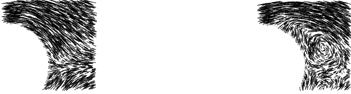
Fig. 8. Development of the boundary layer at the rear of a disk suddenly set in motion
